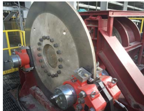
The spring-applied, hydraulically released BSFK 527 brakes act on a 1.9 m diameter disc, mounted to the low-speed side of the drive shaft.
